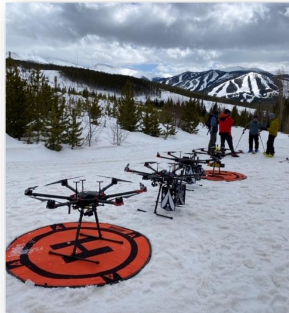
Four separate systems to collect imagery, radar and lidar
