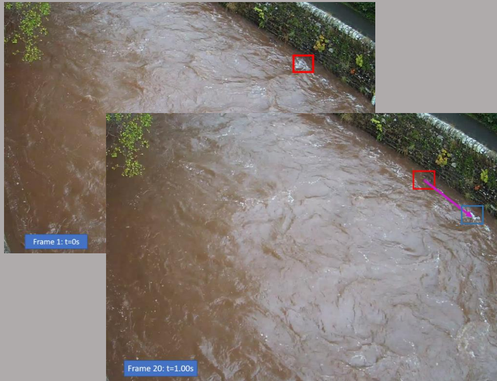
Figure 9: Visible tracers that can be used to track surface velocity between two frames, 1s apart (high flow, roughly around 1.7m/s)
